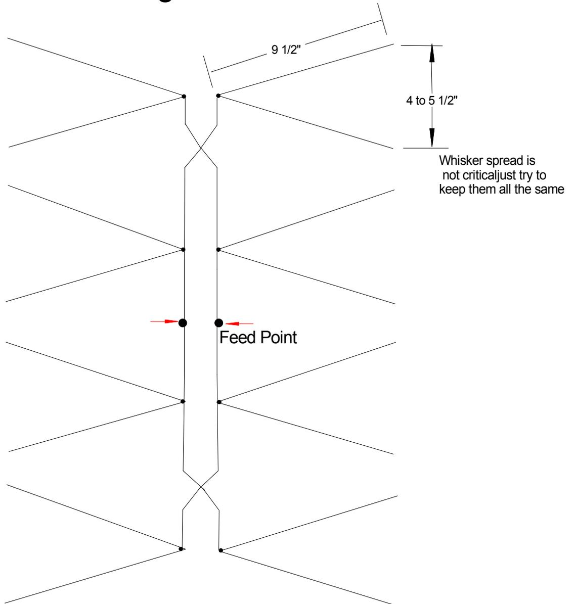
Most any metal will work for the elements. Try to use something near  $\frac{1}{8}$ " diameter and make sure they are free of all coatings and oxidation where they connect to the phase line.
