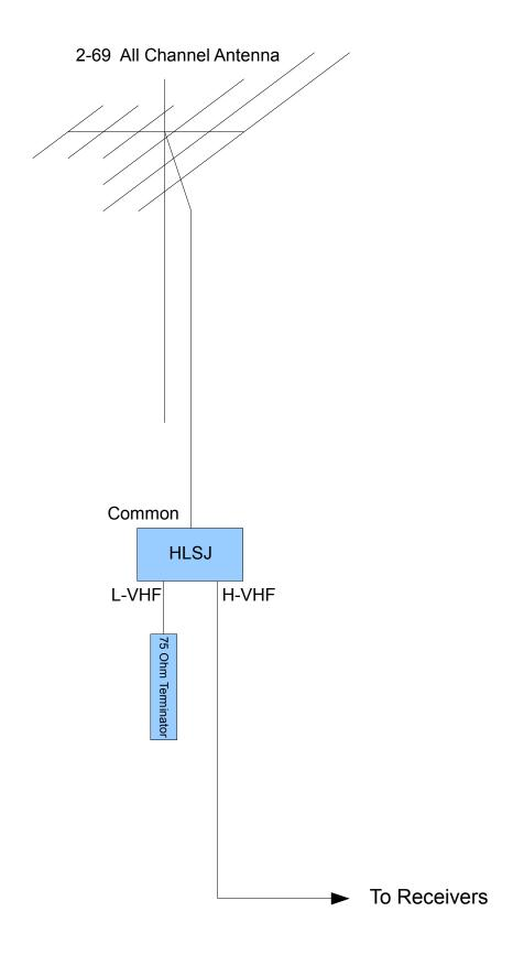
Presuming that the H-VHF port is a high pass filter that does not attenuate UHF frequencies, this arrangement could be expected to attenuate channels in the L-VHF band by 20 dB or more.
