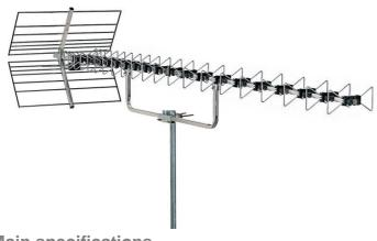
Pre-assembled aerial with F connector and excellent performance: high gain, high directivity and very good return loss. Easy to install and characterised by a highly reliable RF connection. 60mm maximum mast clamp diameter and the design allows good wind loading.
