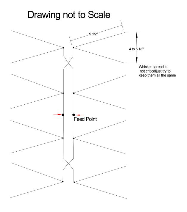
Most any metal will work for the elements. Try to use something near 1/8" diameter and make sure they are free of all coatings and oxidation where they connect to the phase line.
